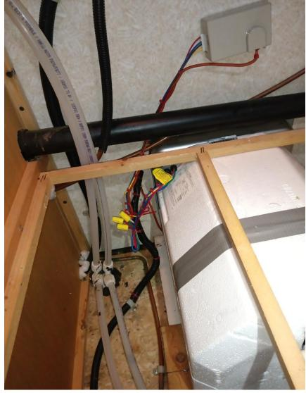
Make sure the bypass valves are not in the bypass condition then fill the HW tank with water and check for leaks. If no leaks continue on. If there are leaks then they need to be addressed. A possible cause is if the Flair-It fittings did not get tightened enough.
